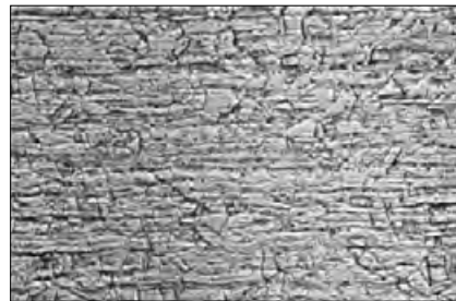
Fig. 1. Stainless steel austenite structure with \delta -ferrite inclusions
