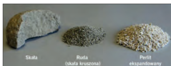
Rys. 4. Różne postaci Perlitu [7] Fig. 4. Different forms of Perlite [7]
