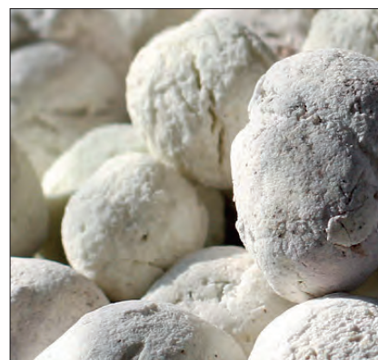
Rys. 2. Kruszywo lekkie Gransil [9] Fig. 2. Gransil lightweight aggregate [9]
