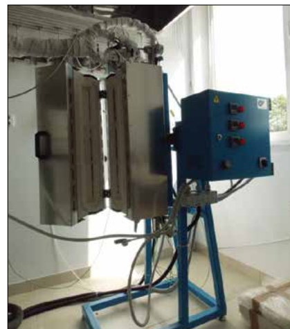
Rys. 5 Mikroreaktor do badania katalizatorów Fig. 5 Microreactor for catalysts investigation
