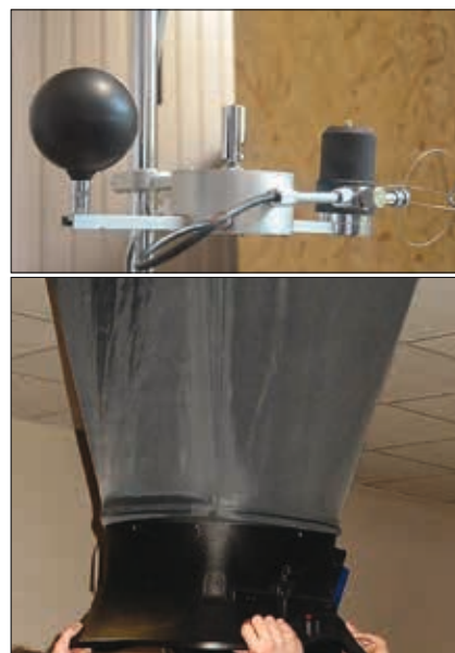
Fig. 5. Measurement module for thermal comfort research (on the left) and balometer for air volume flow rate measurement (on the right)
